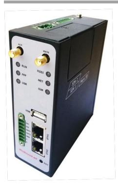
• 3-pin pluggable terminal block with lock for power connector x 1
