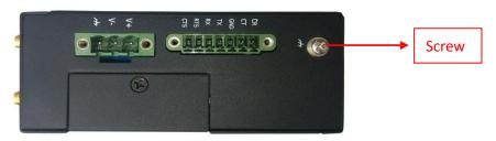
Grounding and wire routing help limit the effects of noise due to electromagnetic interference (EMI). Run the ground
